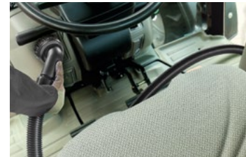
A specific 15-metre vacuum hose can be requested for special needs, for cleaning areas some distance from the vacuum cleaner. It enables the vacuum cleaner to be left outside when cleaning white rooms for instance, or in the agricultural sector to vacuum inside vehicles, leaving the vacuum cleaner on the ground.
