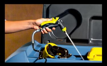
The spray gun has a dual role. During machine maintenance, it facilitates the rinsing of the tanks at the end of the shift, but it can also be used during the work, to moisten stubborn dirt stains and make them easier to remove.
