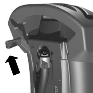
7. Grasp the tube on the rear of the machine
