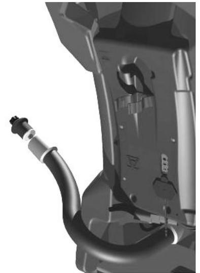
3. Slip off the casing that covers the tank.
